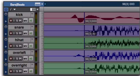
Figure 5. Overhead mics generate late beat triggers
