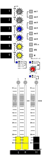
**AUX MASTERS** Each aux mix has a master level control that adjusts the output level to match external equipment, or to trim the monitor, effect or other send without affecting the mix balance. Up to +4dB boost is available above the normal 0dB position.
