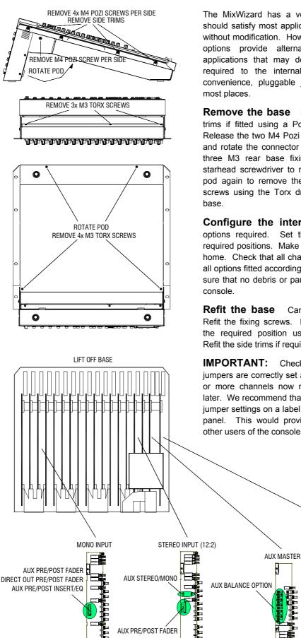
The MixWizard has a versatile architecture which should satisfy most applications you may encounter without modification. However, the following internal options provide alternative settings for those applications that may demand them. Access is required to the internal assemblies. For user convenience, pluggable jumper links are used in most places.
