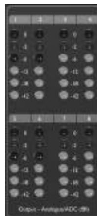
These vertical columns of LEDs indicate the peak signal levels of channels 1-8 in one of two modes, the modes being defined by the fitting of the optional ADC card as follows:-
