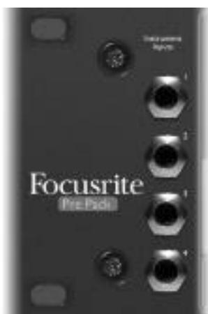
Instrument sources may only be connected via the front panel. Four unbalanced Instrument input connectors are located to the far left of the front panel and are numbered 1-4, correlating to each of the four channels. These connectors are used primarily for connecting low level unbalanced signals such as those from passive guitars and basses, or from active instruments such as keyboards and electro-acoustic guitars.
