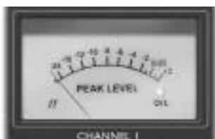
This moving coil meter has been designed to have a very fast reaction time and a slow decay time, and so is perfect
