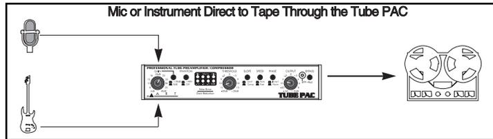
The main application of the Tube PAC is as a microphone preamplifier and compressor. To use the Tube PAC as a mic or line preamplifier only, simply press the Bypass switch to bypass the compression circuitry. Plug any microphone directly into either input and set the input and output controls to provide an appropriate level into the next stage of your system.
